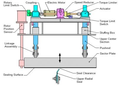
Figure 4. Diagram of LVP's Adjustable Seal Design
