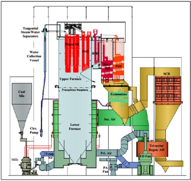
Figure 2. Cut-away of LVP's Pulverized Coal Boiler
