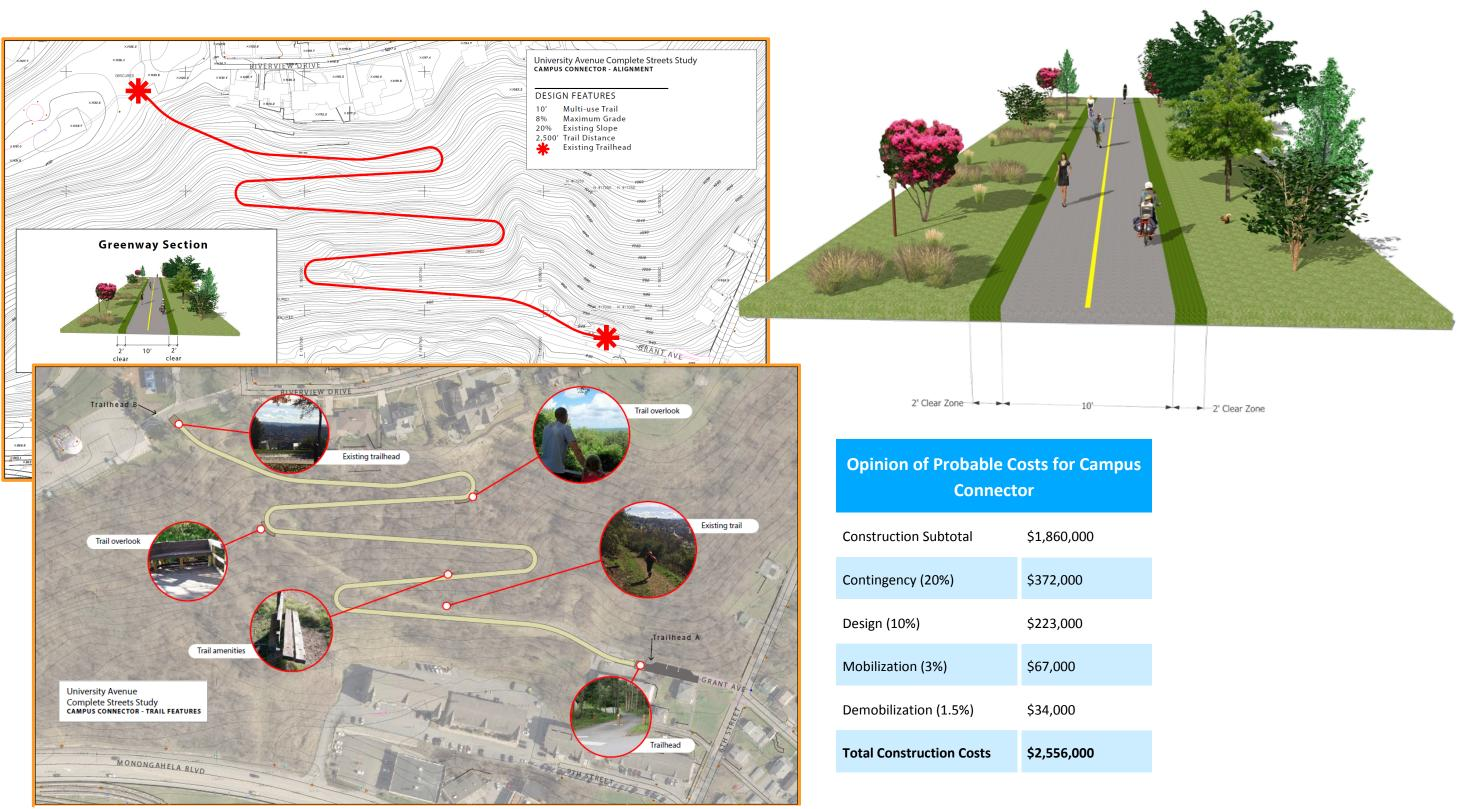
Figure 28. Campus Connector Path (top); Features (bottom); and cross-section
