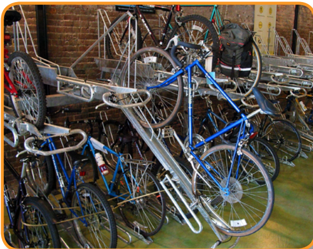
Figure 2-8: Articulated upper tray (photo: Heath Maddox)
